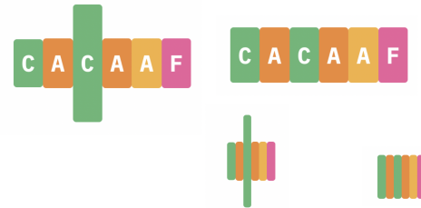
Figure 1. The SNAC visual encoding for neural network architectures. This model has a two convolutions, each followed by an activation, and concludes with an average pooling layer and a fully connected layer. Each block represents a layer in a sequential CNN. Color encodes the type of layer, while width can be used to encode a numeric attribute such as tensor width. Additional attributes can be made available via tooltip if SNAC is deployed in a web application. SNAC functions at several different sizes and fixed widths.
